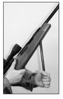
IN ADDITION TO THE SAFETY CATCH THAT DISABLES THE TRIGGER MECHANISM, THIS RIFLE HAS A 'SAFETY LOCK' THAT PROVIDES A FULL MECHANICAL LOCK TO THE SLIDING BREECH AT THE END OF THE COCKING STROKE. THIS SAFETY DEVICE GIVES ADDITIONAL SECURITY WHEN INSERTING A PELLET, HOWEVER THE USER IS STILL ADVISED TO KEEP HOLD OF THE COCKING ARM AS ILLUSTRATED ABOVE.
