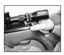
RELEASE THE SAFETY CATCH BY PUSHING THE BUTTON IN FULLY. THE RIFLE IS NOW READY TO FIRE. THE SAFETY CATCH CANNOT BE RE-ENGAGED WITHOUT RE-COCKING THE RIFLE SO DO NOT RELEASE THE SAFETY CATCH BEFORE YOU NEED TO.
