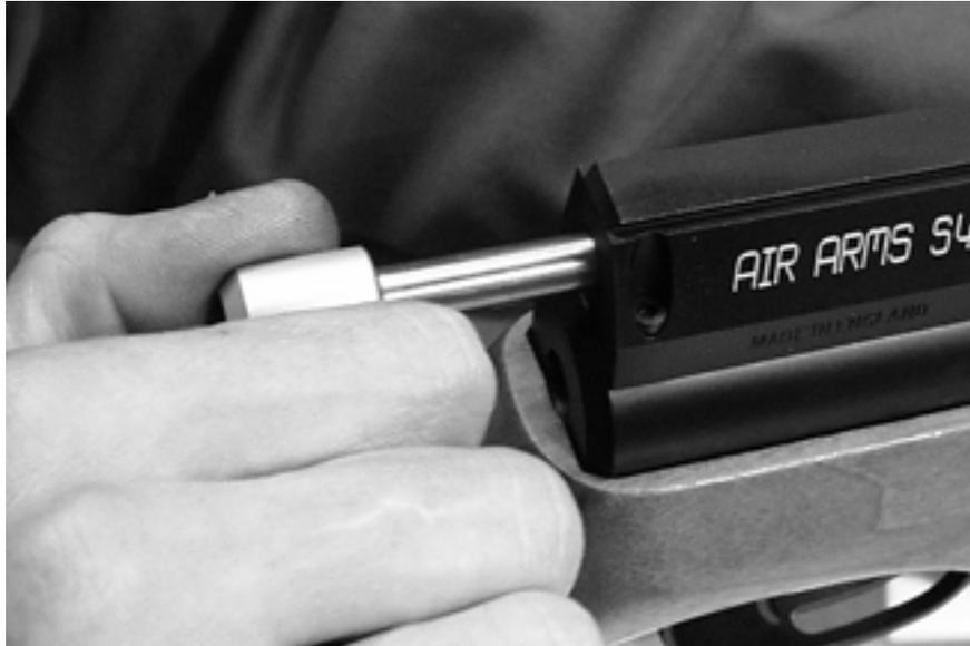
NOTE ! IT IS VERY IMPORTANT THAT THE LOADING BOLT IS PULLED BACK TO THE CORRECT POSITION IN ONE POSITIVE MOTION. THE MAGAZINE INDEXES TO THE NEXT PELLET POSITION AS THE BOLT IS RETRACTED AND IT IS POSSIBLE FOR A PARTIAL INDEX IF THE BOLT IS NOT PULLED BACK FULLY.
