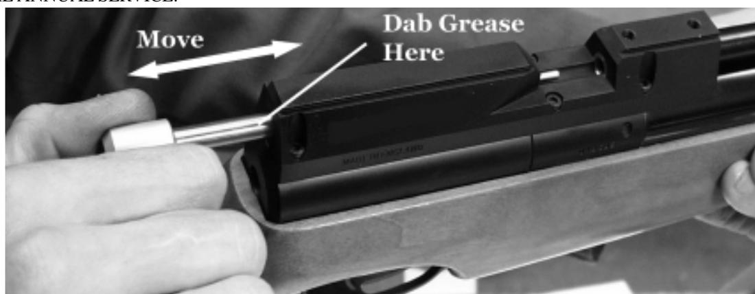
APPLY A SMALL DAB OF GREASE ON THE LOADING BOLT AND WORK-IN BY MOVING THE BOLT FORWARDS AND BACKWARDS. WIPE OFF EXCESSIVE GREASE. PREFERRED GREASE IS 'NAPIER G95 GUN GREASE'
