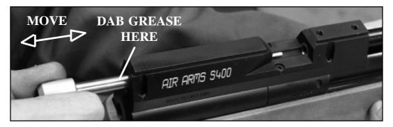
APPLY A SMALL DAB OF GREASE ON THE LOADING BOLT AND WORK-IN BY MOVING THE BOLT FORWARDS AND BACKWARDS. WIPE OFF EXCESSIVE GREASE. PREFERRED GREASE IS 'NAPIER G95 GUN GREASE'
