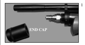
REMOVE END CAP BY TURNING ANTICLOCKWISE.
